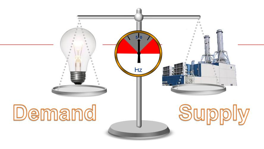
When supply is increased to match demand, frequency recovers to 50 Hz
